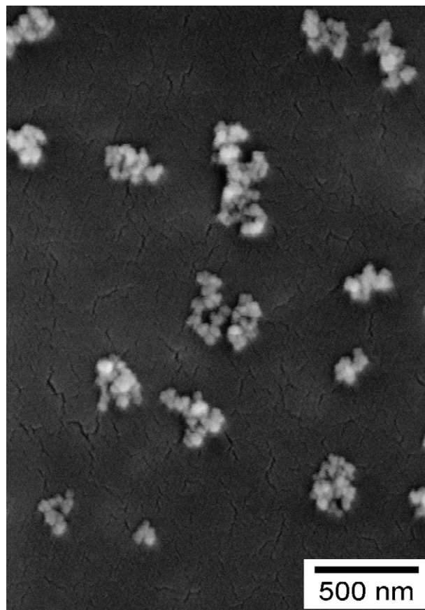
Fig. 1. SEM picture of a suspension of HDK HKS D silica in water. The primary silica particles of diameter 15–20 nm are forming aggregates of 100–200 nm size.
